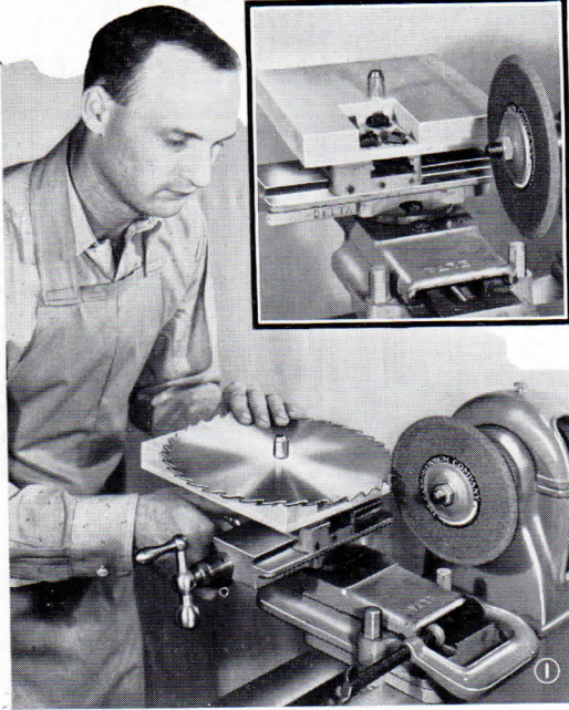
Above, simple automatic method of gumming and grinding circular saw blades. Below, dressing wheel and grinding backs of teeth.
